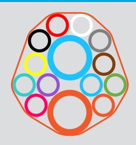
Höhle microducts are designed for long term protection of fiber optical cables. Direct Bury (DB) type of microducts are thick wall products that attain their mechanical robustness and functional performance through their intrinsic thick walls and need no further protection at underground installations.
